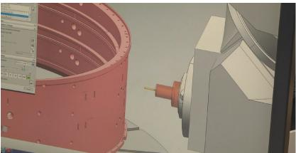
"The strength of NX is that it is very easy to compare the model of the raw material prior to machining with the finished product. After the programming of any tool path, NX gives a visual representation of the material that has been removed and any that is left. This means that we are constantly up to date with the amount of metal the program will remove and also the amount remaining."
